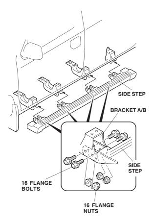
9. Adjust the location of the left side step so there is even clearance between the side step and body, then tighten the flange bolts you installed in step 7. Torque 14 flange bolts to 27 N·m (20 lbf·ft), and the one remaining flange bolt to 7 N·m (5 lbf·ft) as shown.
