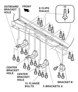
Install three brackets A and one bracket B to the body using 15 flange bolts. Thread the flange bolts in about 3 to 4 threads. When installing brackets A, use the outboard bracket holes for the front bracket, and the center bracket holes for the center and rear brackets. 8. Install the side step to the brackets using 16 flange bolts and 16 flange nuts. Thread the nuts on about 3 to 4 threads.
