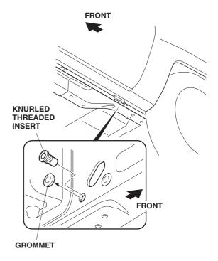
Screw the knurled threaded insert onto the mandrel of the tool as shown.
