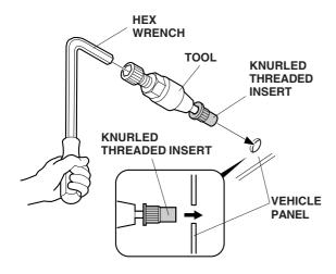
4. Holding the tool with the hex wrench, turn the 27 mm wrench clockwise and install the knurled threaded insert in the vehicle panel.
