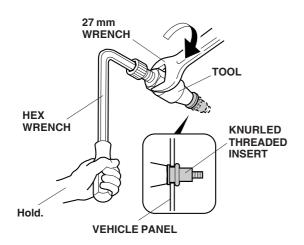
5. Remove the tool from the knurled threaded insert by turning the hex wrench counterclockwise.
